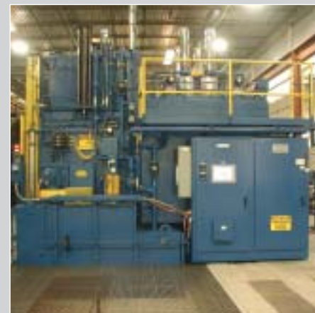
UBQ with BatchMaster PC control system.
