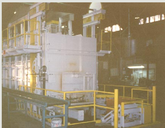
Pusher Tray Solution Furnace
