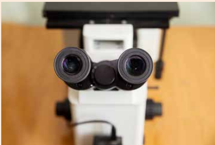
A metallograph, as it was known then, is a glorified microscope designed to view polished and etched metallurgical samples, micros, of metal at high magnification.
