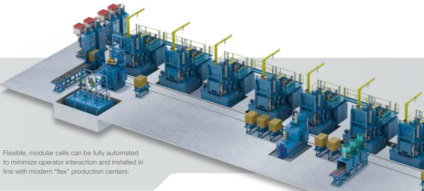
Flexible, modular cells can be fully automated to minimize operator interaction and installed in line with modern “flex” production centers.
