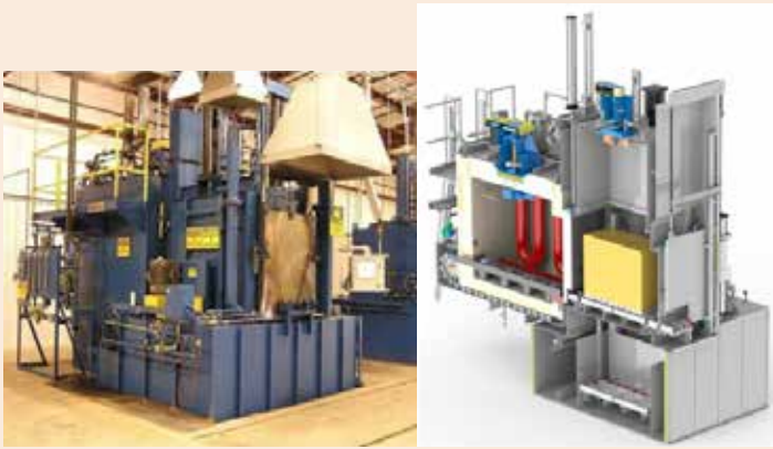
Figure 3: UBQ Integral quench batch furnace. (Courtesy: AFC-Holcroft.com)
