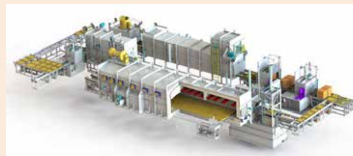
Figure 2: Complete three-row pusher layout, furnace, wash, temper and material handling. (Courtesy: AFC-Holcroft.com)
