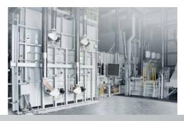
Patented water injection system provides quench severity similar to water quench
