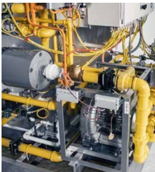
AutoGen standard on AFC-Holcroft EZ ® Generator
