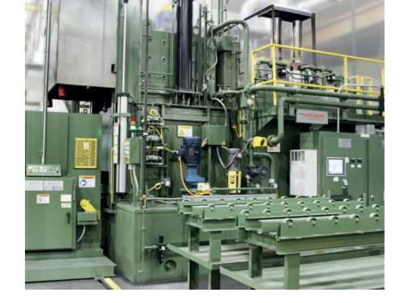
External rear handler drive can provide automatic transfer of workload from furnace to quench tank after completed cycle.
