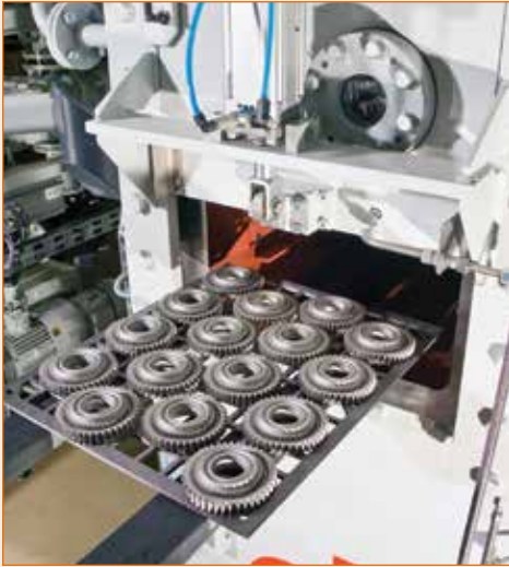
Figure 1: SyncroTherm® load arrangement.
