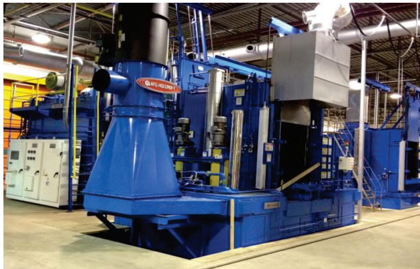
Fig. 2 — Universal batch quench austemper furnace (914 × 1829 × 1422 mm) used at Zanardi Fonderie S.p.A. to study heat treated properties of cast iron and austempered ductile iron. Three chambers enable transferring product to a salt-quench tank under a protective atmosphere.
