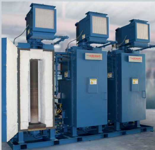
Hinged retort access door for easy retort maintenance
